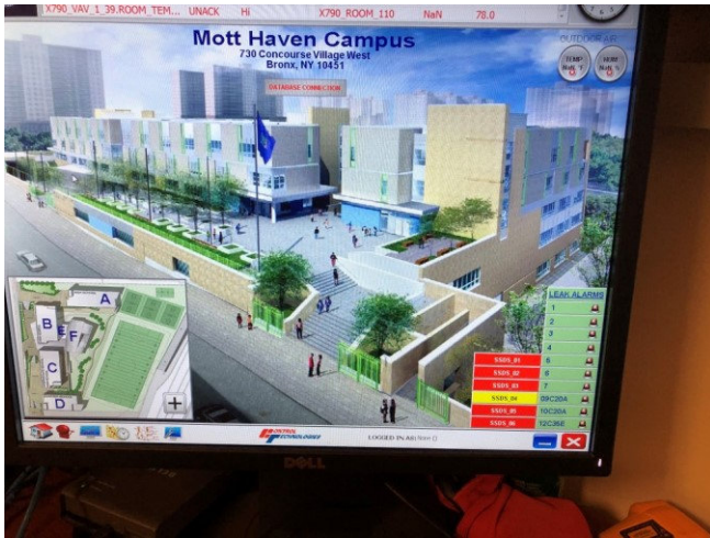
Photo 1: View of BMS, reportedly not operating correctly.
