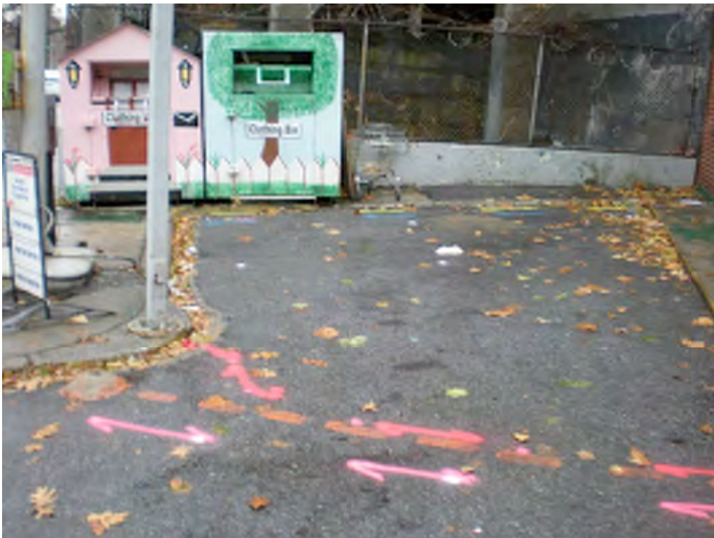
Figure 2 – Designated utilities near the eastern side of the main building. No anomalies consistent with USTs were found in this area.
