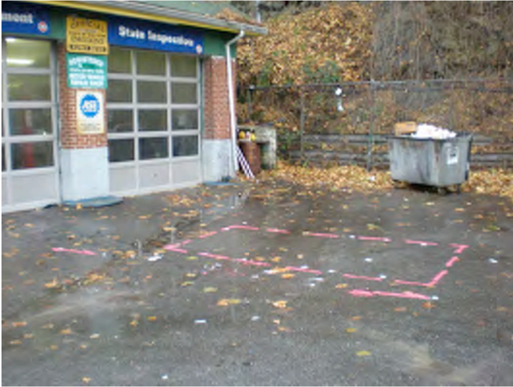
Figure 1 – Non-metallic anomaly (pink rectangle) near the northern side of the main building. Note the unknown utility line (pink arrows) designated near the anomaly.
