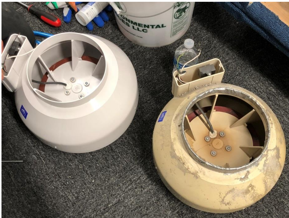
Photograph 8 – View of replacement blower B-3 (left) and inoperable blower (right). Taken on 07/26/2018.
