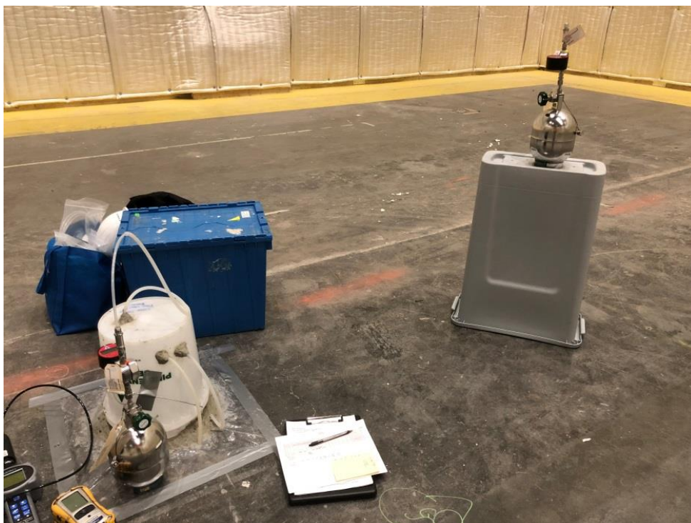
Photo 4 – View of co-located soil vapor and indoor air sample at SVMF -04, facing south. Taken on 05/24/2018.
