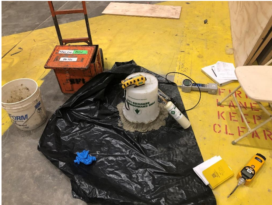
Photo 3: View of helium tracer test being performed on soil vapor point SVMF-07, facing north. Taken on 06/22/2019.
