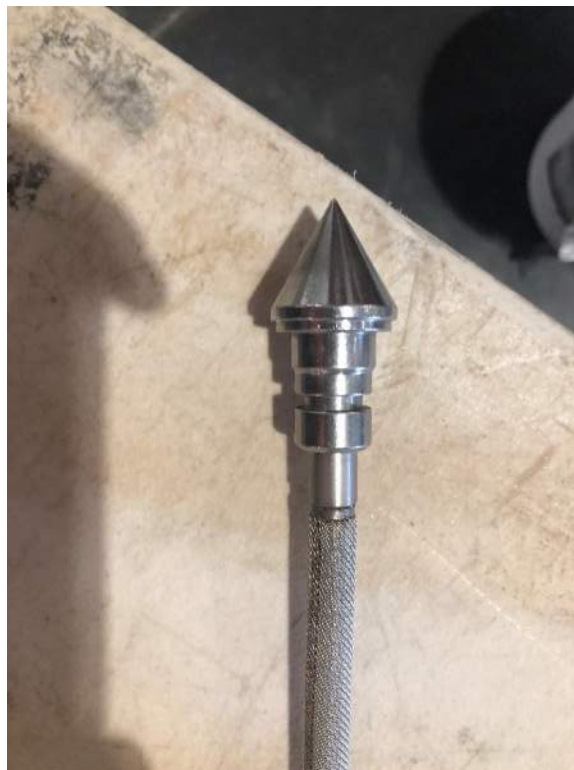
Photo 2: View of Geoprobe® soil vapor implant anchor attached to stainless steel screen prior to installation.
