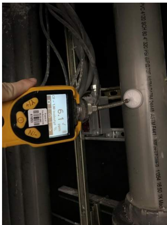
Photo 2: Collection of VOC readings from the SMD Riser Pipe
