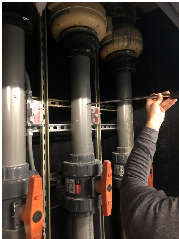
Photo 1: View of velocity gauging using a TSI Velocalc at the blower system manifold closet.
