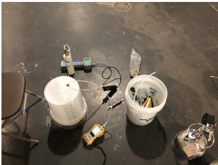
Photo 2: View of Helium shroud test prior to sample collection.
