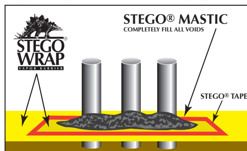
FIGURE 4: MULTIPLE PIPE PENETRATION SEALING
