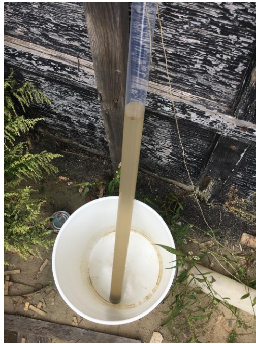
Photo 5: Bailer used to visually inspect well water for remaining product after VEFR
