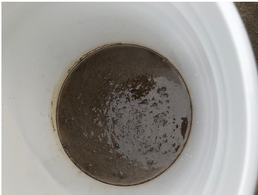
Photo 4: Fluid collected in knockout pot
