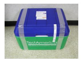
F. Close cooler, place signed and dated Custody Seals over opening. Tape over the Custody Seal and seal cooler securely. Fill out overnight shipping waybill and attach to the top or handle of the cooler. Attach Saturday delivery stickers if needed. Ship according to DOT regulations.
