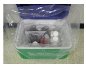
B. Wipe outside of bottles and put glass in individual bubble bags & seal. Place bottles & the temperature blank into cooler. Leave room for ice in between bottles & on top.
