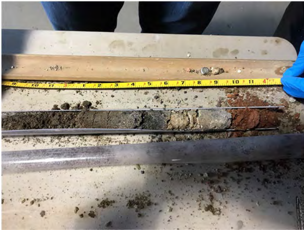
Photo 19: SB-7 (0-5') in WC-3 – Fill containing brick, concrete, and trace coal.
