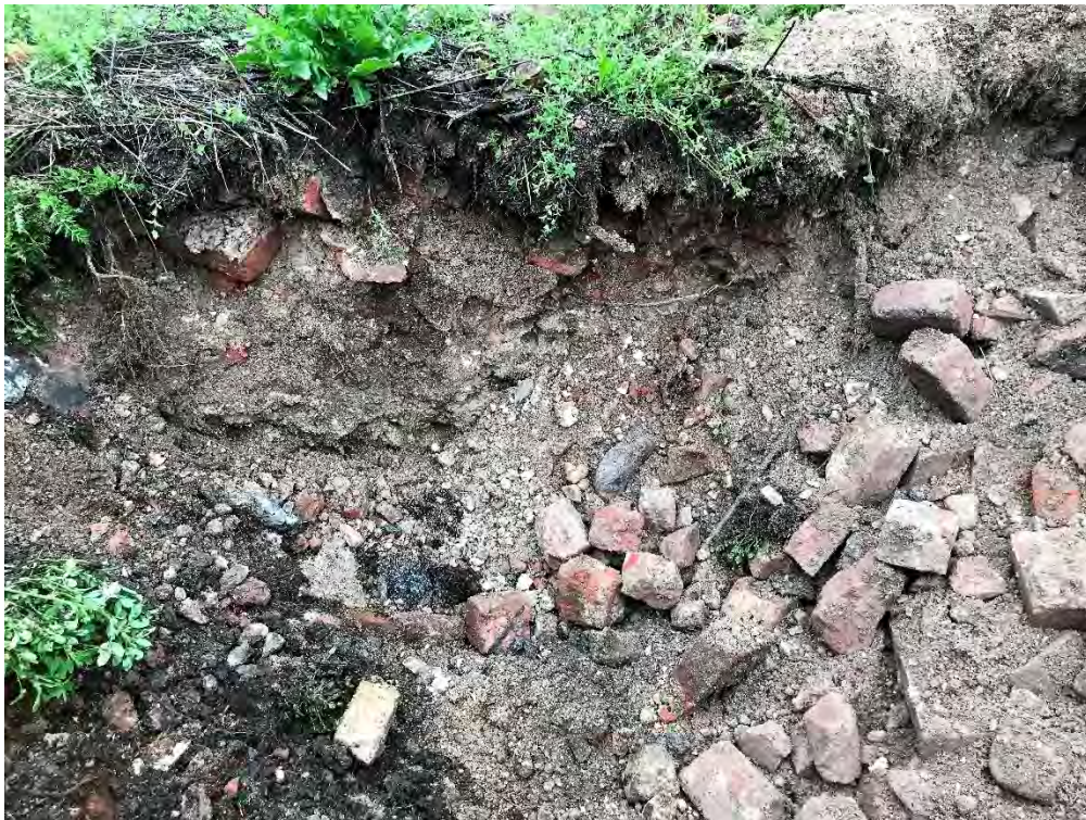
Photo 4: TP-3 in WC-5 – Fill material consisting of brick, concrete, and metal debris.
