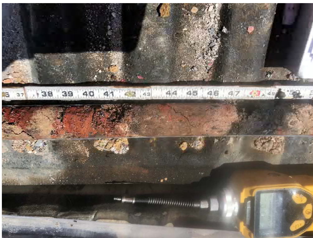
Photo 17: SB-6 (0-5') in WC-2 – Fill containing brick, concrete, and trace coal/slag.
