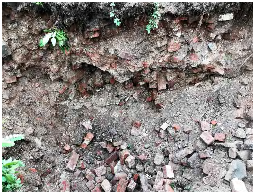
Photo 2: TP-2 in WC-5 - Fill material consisting of brick, concrete, and metal debris.
