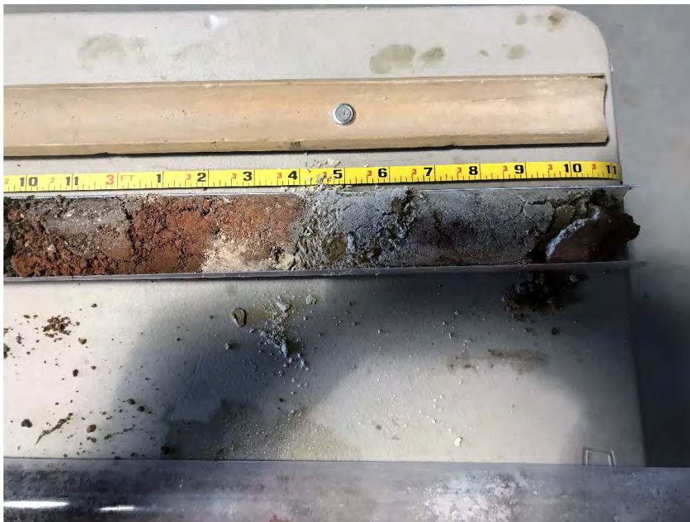
Photo 12: SB-1 (5-10') in WC-1 – Fill containing brick and concrete.
