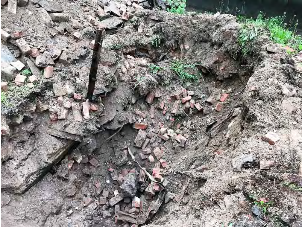
Photo 3: TP-1 in WC-5 – Fill material consisting of brick, concrete, and metal debris.
