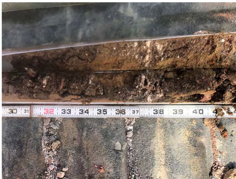
Photo 16: SB-5 (15-20') in WC-2 – Fill containing brick, concrete, and trace coal/slag in a brown coarse-to-medium sand matrix.
