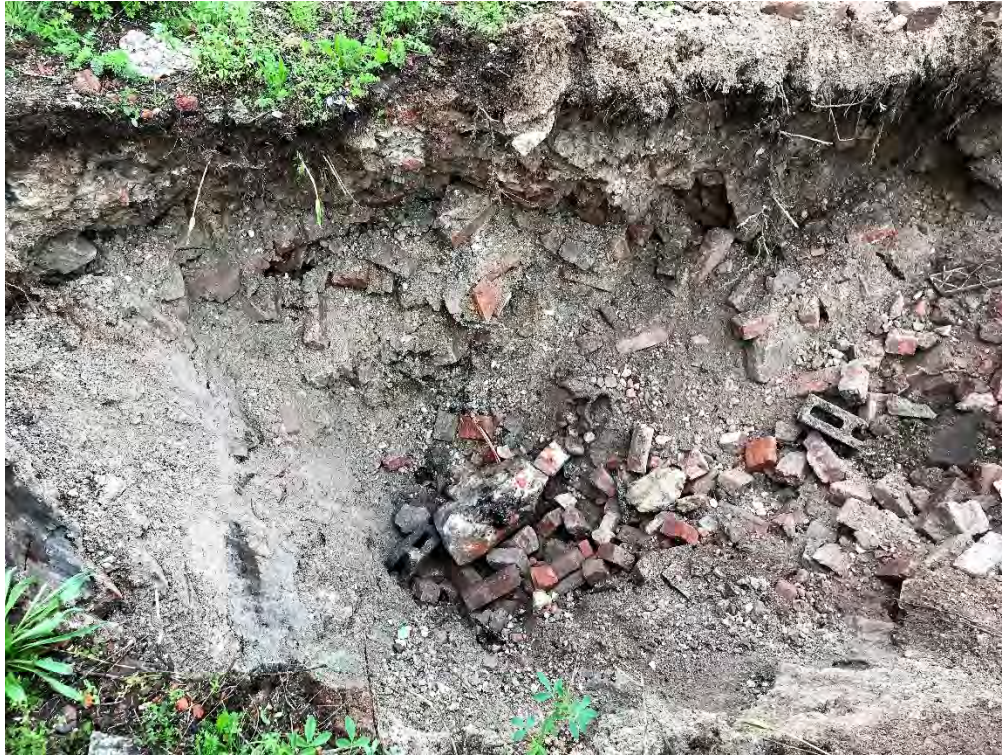
Photo 5: TP-4 in WC-5 – Fill material consisting of brick, concrete, and metal debris.
