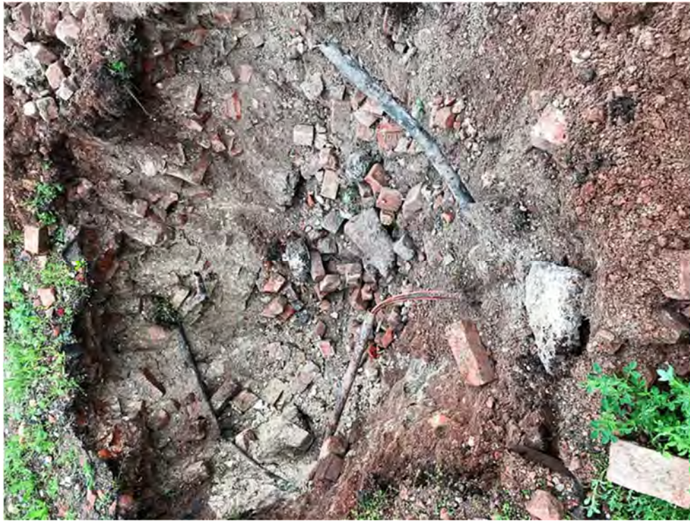
Photo 11: TP-9 in WC-4 – Fill material consisting of brick, concrete, and metal debris.
