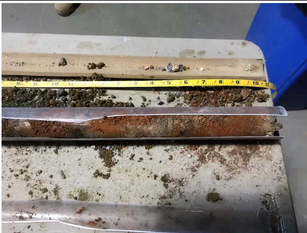
Photo 18: SB-8 (5-10') in WC-3 – Fill containing brick, concrete, and trace slag.
