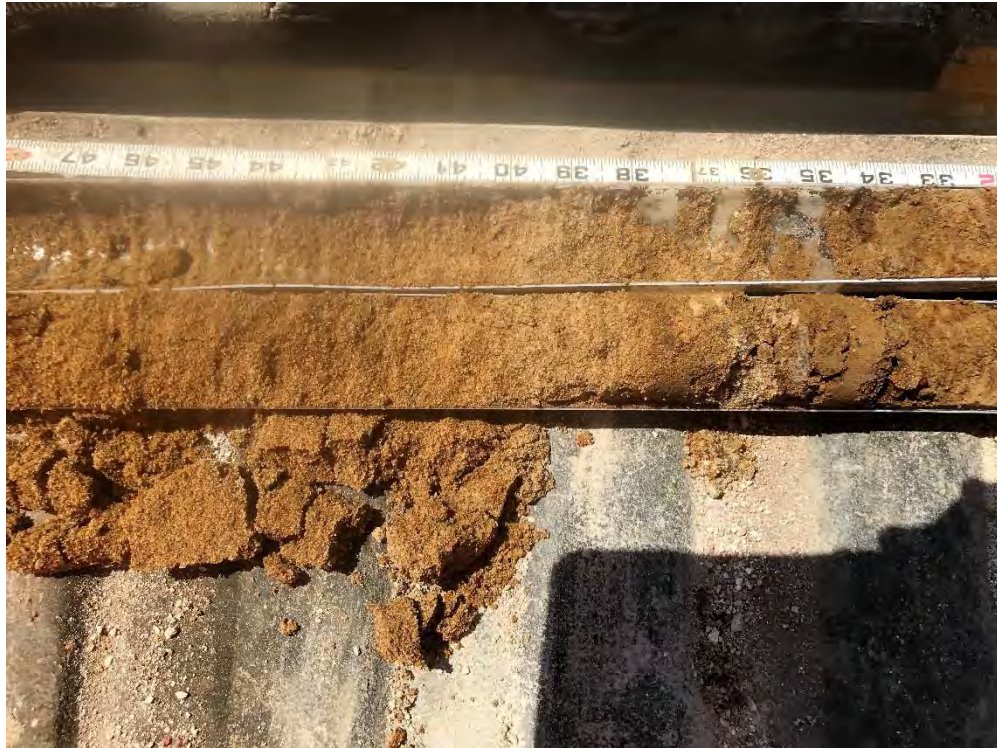
Photo 14: SB-4 (10-15') in WC-2 – Tan/brown coarse-to-medium sand native soil.
