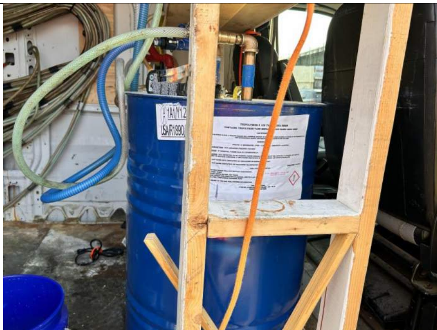
Photo 1: View of Tripolymer® 105 Tank Media Resin in container inside Endeavour's support vehicle (facing north).
