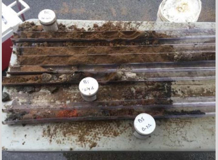
PHOTO 2: Soil boring cores from B-5
