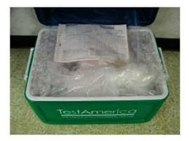
E. Close outer bag, compress excess air out of bag, twist top and knot. If necessary, use more bubble wrap to fill the dead air spaces. Place chain of custody (COC) and other paperwork in plastic bag and seal. Place on top of cooler.
