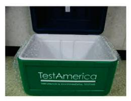
A. Line cooler with bubble wrap and large plastic bag. Use absorbent pad inside the bag if bottles contain preservatives.
