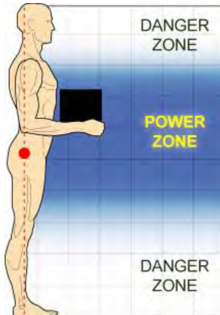
Figure 1: Lifting Power Zone
