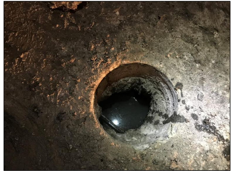
Photograph 2: Groundwater encountered immediately beneath the Site building cellar slab at soil boring RI-SB-11.
