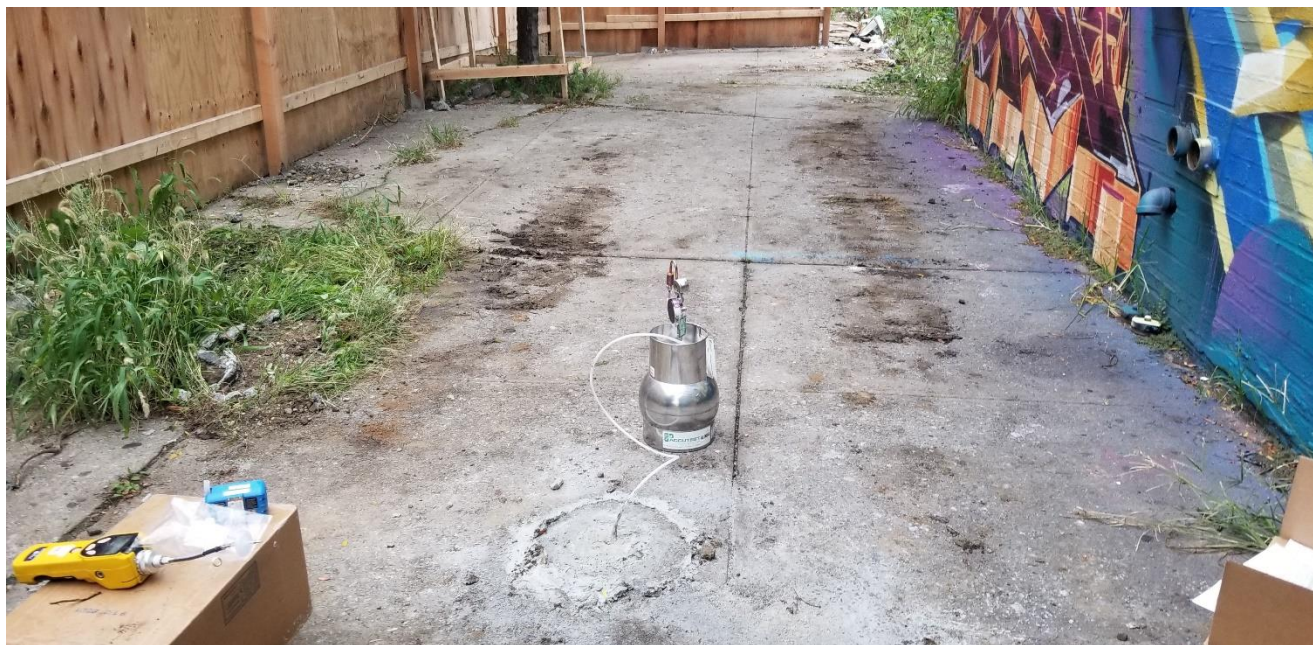
Sampling temporary soil vapor points RI-SV-03 in the Westchester Avenue sidewalk.
