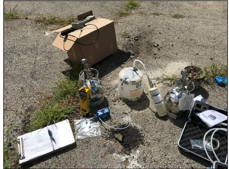
Photograph 6: Purging and screening at temporary soil vapor point RI-SV-07 prior to sample collection.
