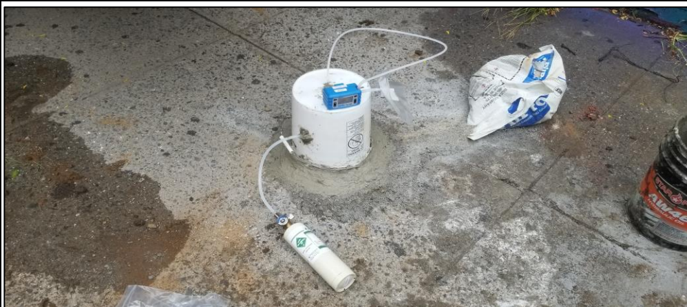
Photograph 3 - Purging vapors prior to sampling at temporary soil vapor point RI-SV-03.
