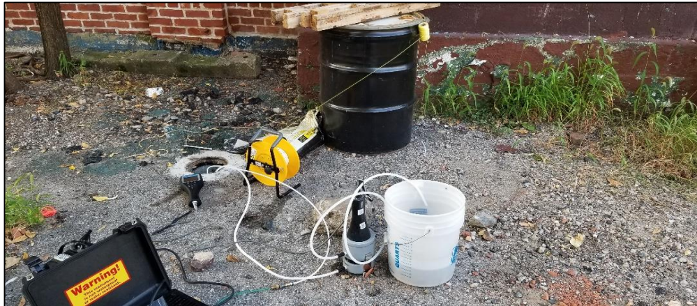
Photograph 1 - Sampling at groundwater monitoring well RI- MW-05 on the north- central portion of the Site.
