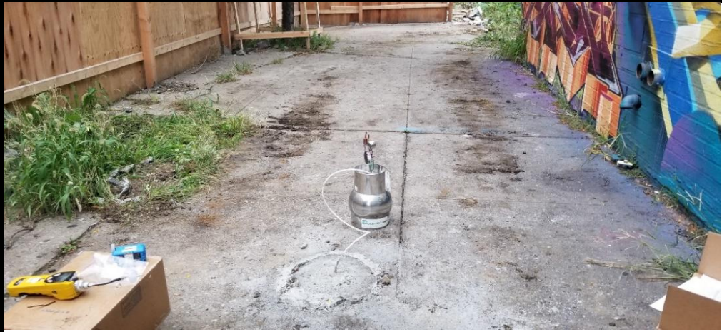
Photograph 1 - Sampling of soil vapor point RI-SV-03 on the south-central portion of the Site within the Westchester Avenue sidewalk.
