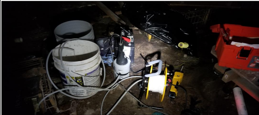
Photograph 2 - Sampling at groundwater monitoring well RI- MW-04 on the eastern portion of the Site in the Site building cellar.
