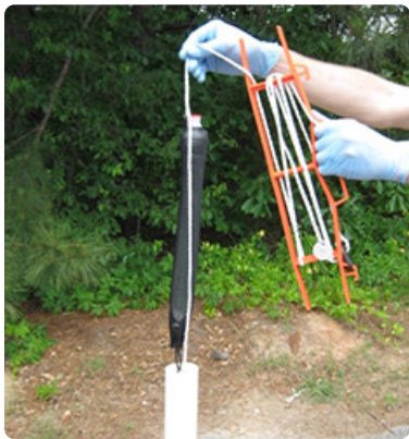
Figure 7 – Example passive diffusion sampler.
