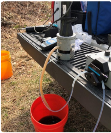
Figure 1 - Image of groundwater with suspended colloidal carbon poured into a bucket. The groundwater appears quite dark but once tested was safe to send to an analytical laboratory for accurate samples.
