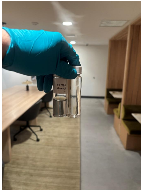
Photo 2: View of purged groundwater from RMW14 compared to the PetroFix 50 milligrams per liter (mg/L) standard.
