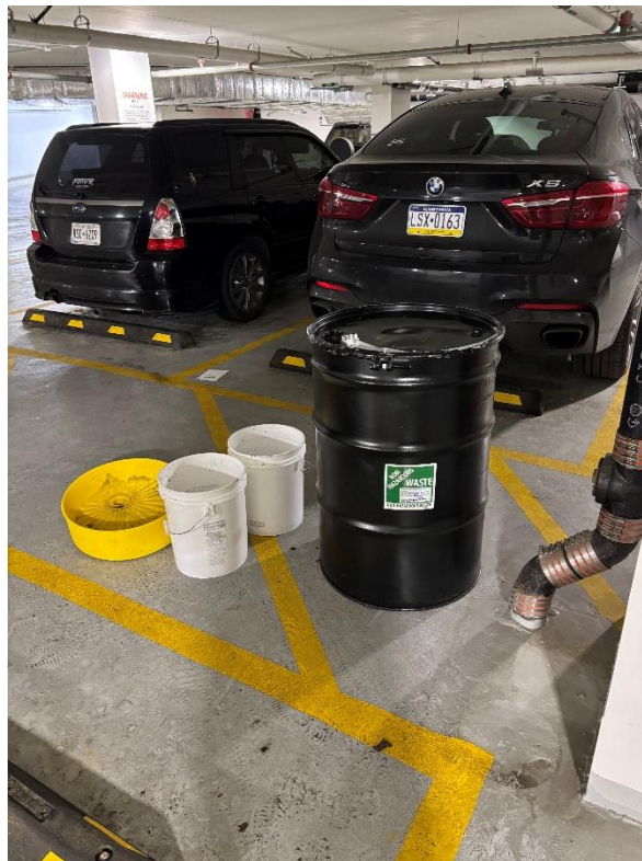
Photo 2: View of purged groundwater stored in labeled 55-gallon drum.
