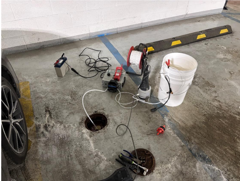
Photo 1: View of groundwater sampling at monitoring well RMW09.
