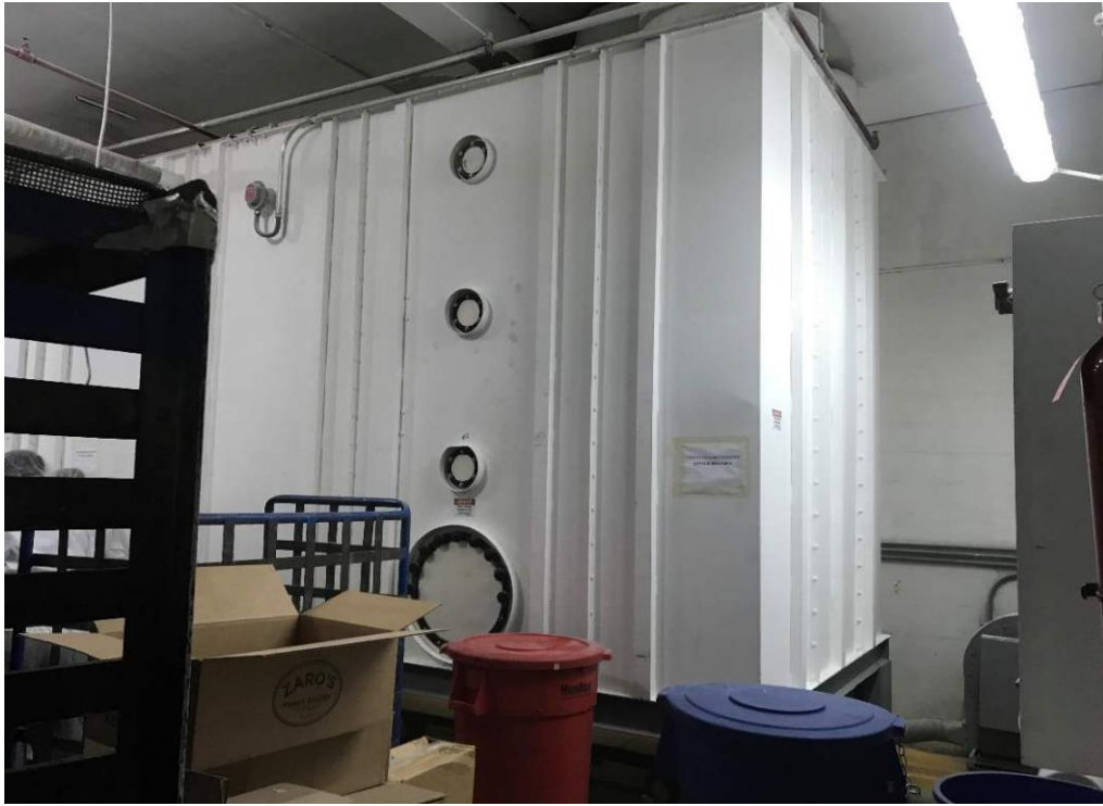
Photo 9: 80,000-pound flour silo located on the ground level.
