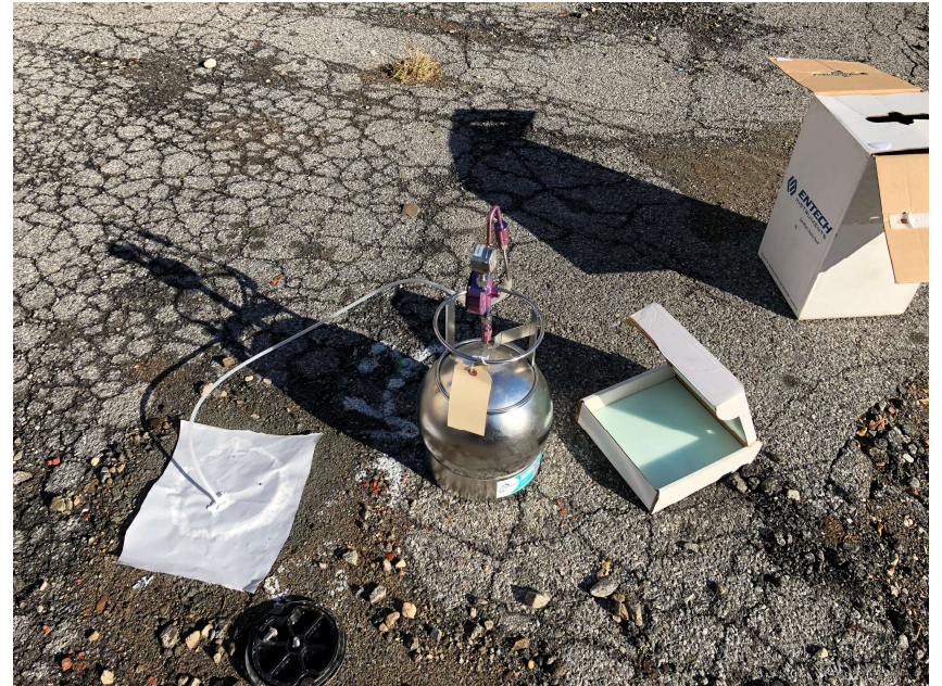
Typical Soil Vapor Sampling
