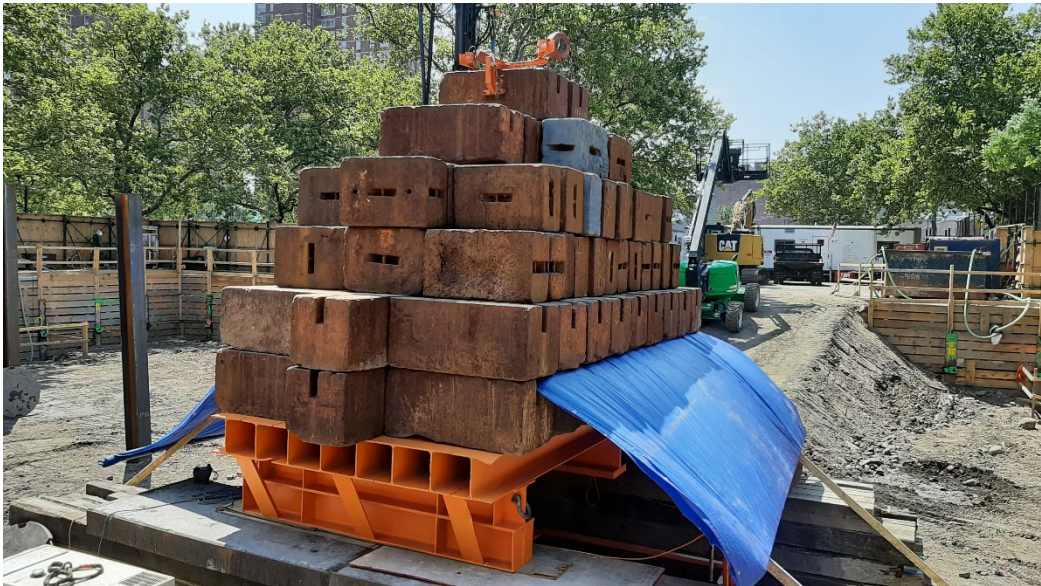
Photo 3: View of completed pile stress test load by end of day.
