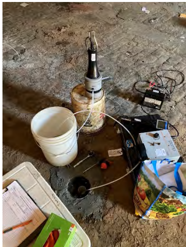
Photo 1: View of groundwater purging.
