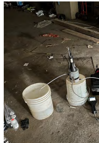
Photo 2: View of Horiba setup and stabilization measurements collection during low flow groundwater sampling.
