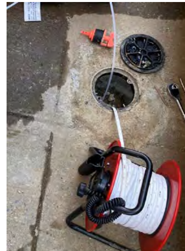
Photo 2: View of monitoring drawdown during low flow groundwater sampling.
