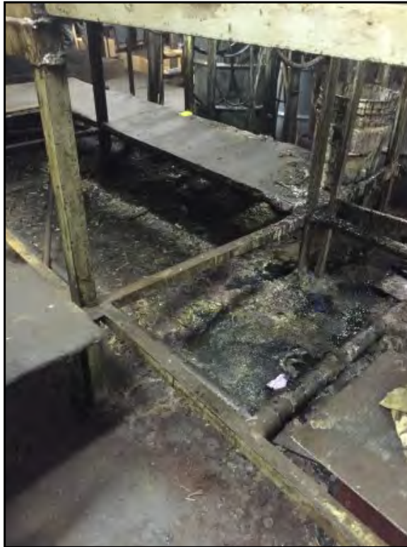
Staining observed beneath ovens located within plastic manufacturing facility.
