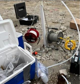
Photo 3: View of groundwater sampling at MW-1X.
