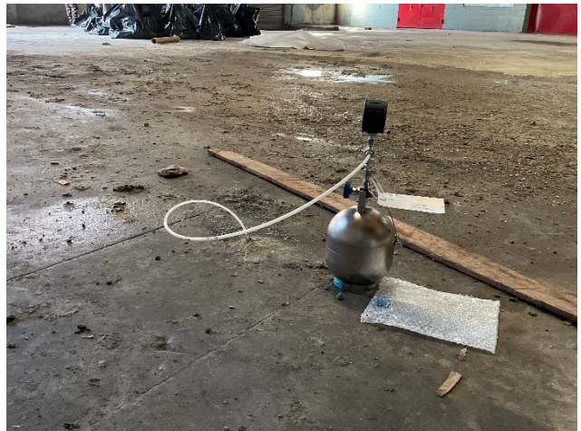
Photo 4: SS-01 soil vapor collection setup
