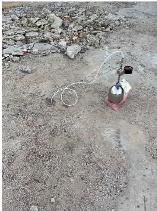
Photo 2: Soil vapor sample collection.
