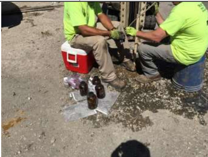
PHOTO 21: Ground water sampling GW-4
