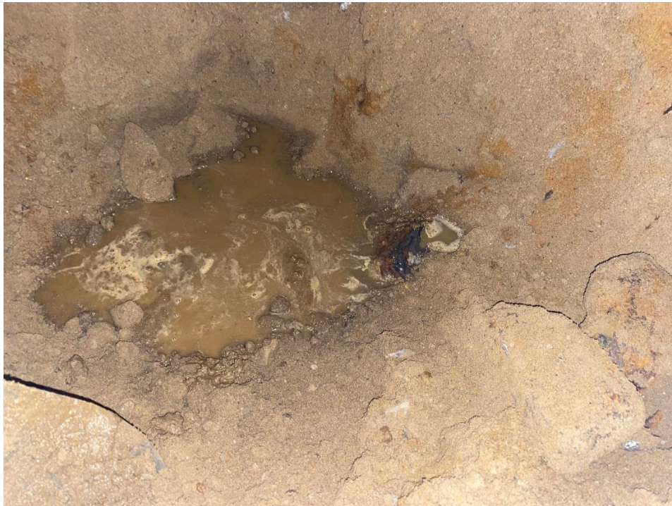
Large Test Pit within the Interior Parking Area, showing leaking UST.
