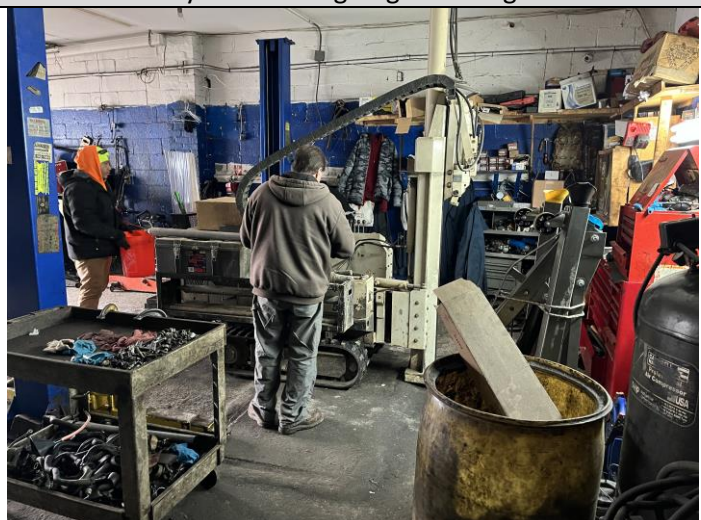
PHOTO 6: Soil Boring B-1 using Geoprobe drill rig
