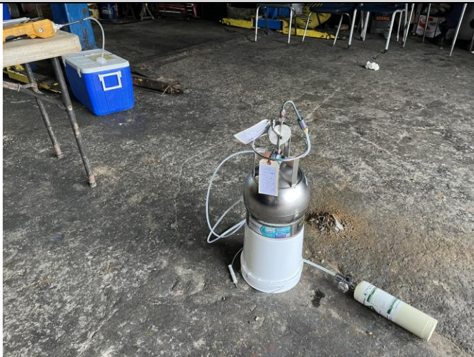
PHOTO 11: Soil Vapor Sample SV-2
