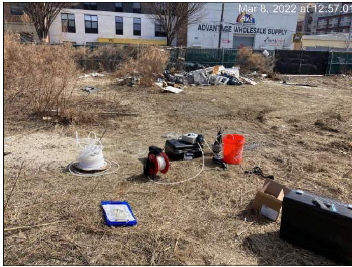
Photograph 9. Groundwater purging and sampling at location TW-02 on the eastern portion of the Site.
