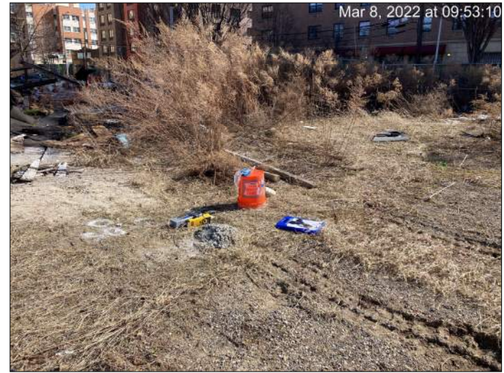
Photograph 6. Vapor point seal check with helium and helium meter prior to sampling at location SV-02 on the eastern portion of the Site.
