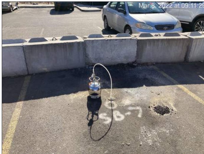
Photograph 7. 6-liter vacuum canister utilized for collection of soil vapor sample SV-06 on the central portion of the Site.
