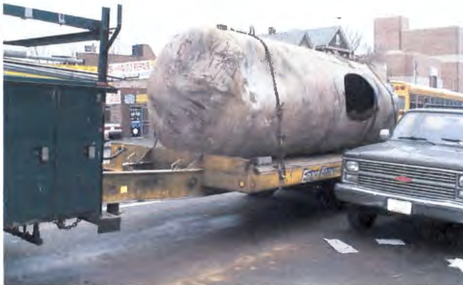
4,000-GALLON GASOLINE TANK TRANSPORTED
