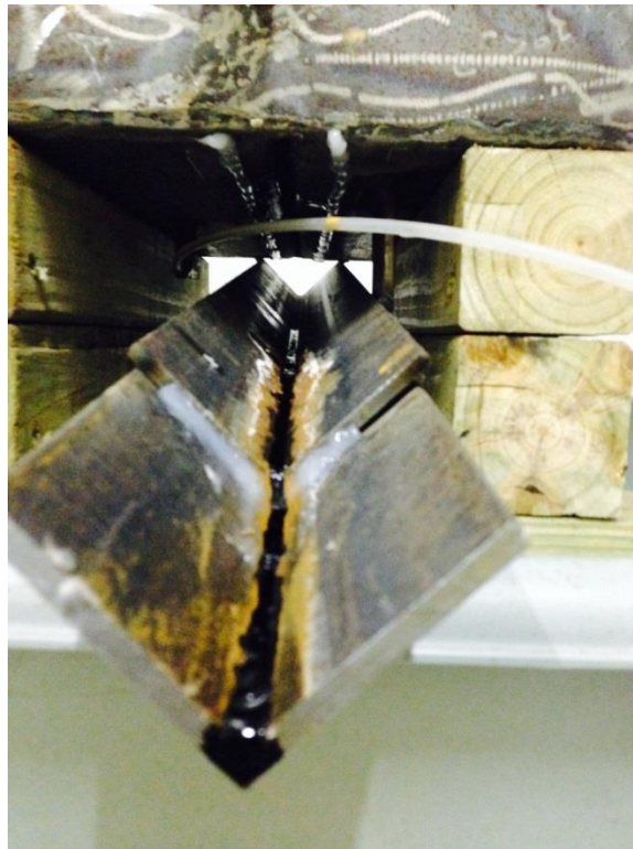
Fig. 4 – Catch Angle showing DNAPL Discharge from Joint.
