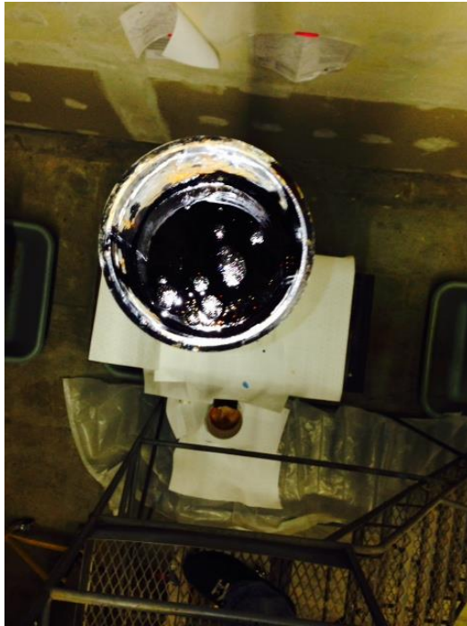
Fig. 7 – Top of Standpipe filled with DNAPL.
