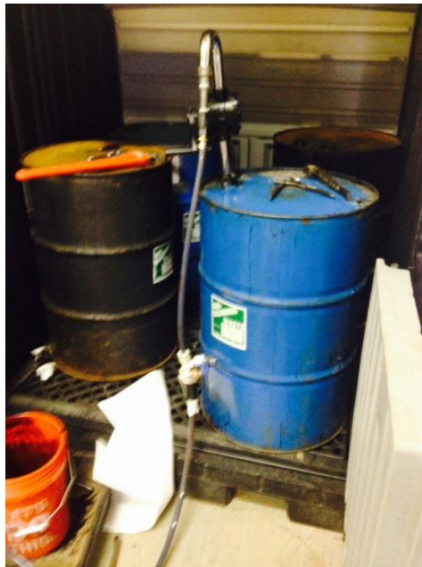
Fig. 3 – Pump Setup in Drum filled with DNAPL.
