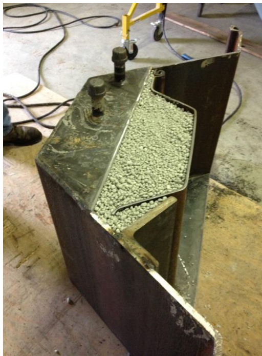
Fig. 2 – Barrier Cell Enclosure filled with AquaBlock 3070 SW.
