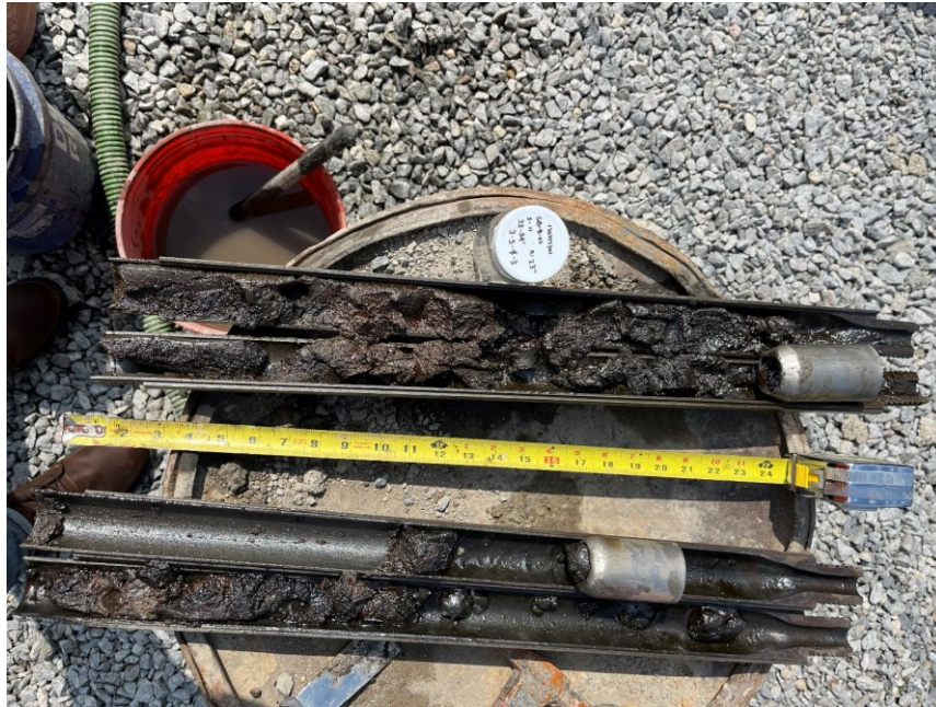
Photo 1: Soil/fill recovered from geotechnical boring GB-B-02
