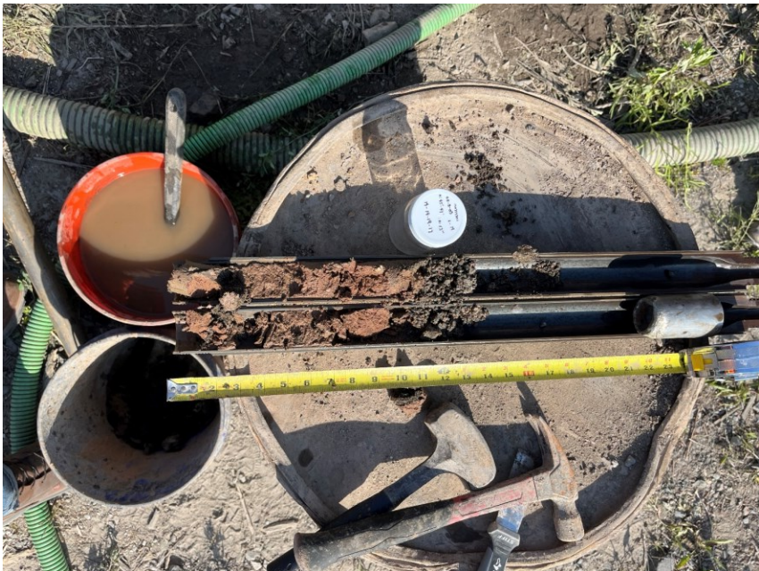
Photo 1: Soil/fill recovered from geotechnical boring GB-D-03
