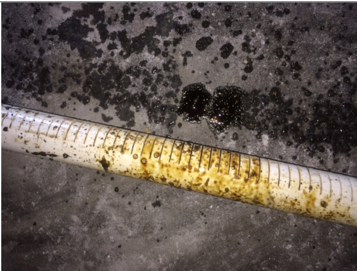
4. Temporary well screen from TMW4
