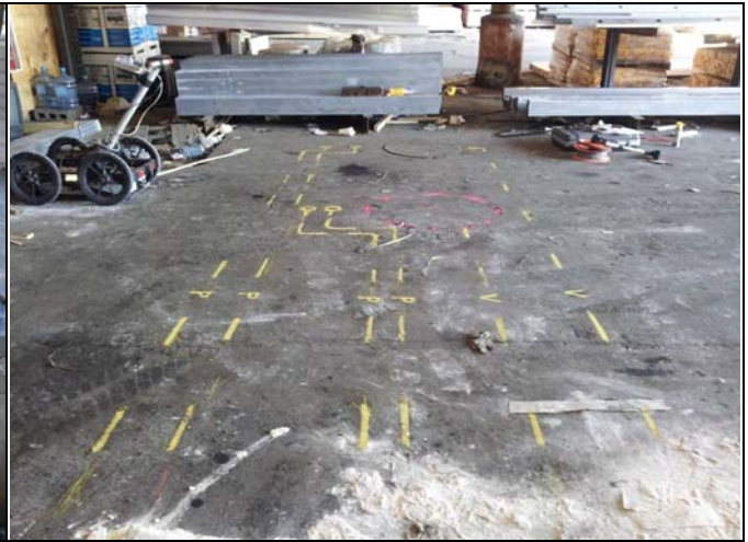
Two USTs and associated piping, facing east
