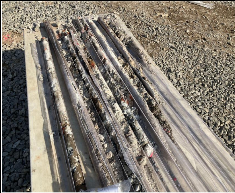
Photo 3: View of utility trench soil borings.
