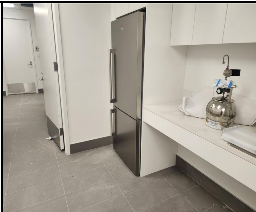
Photo 3: View of a summa canister collecting indoor air sample.
