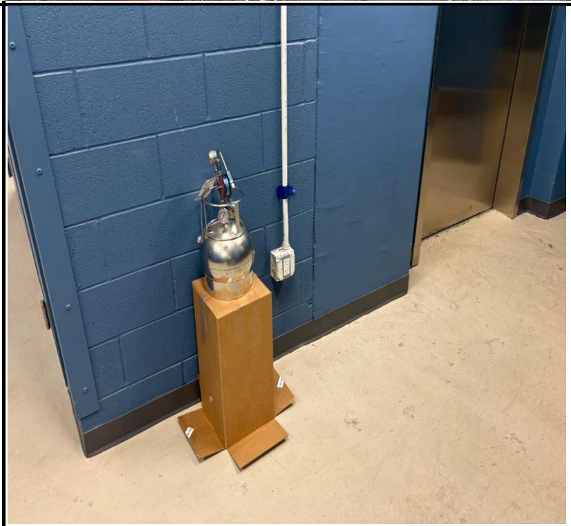
Photo 2: View of indoor air sample location A2-1A-5.
