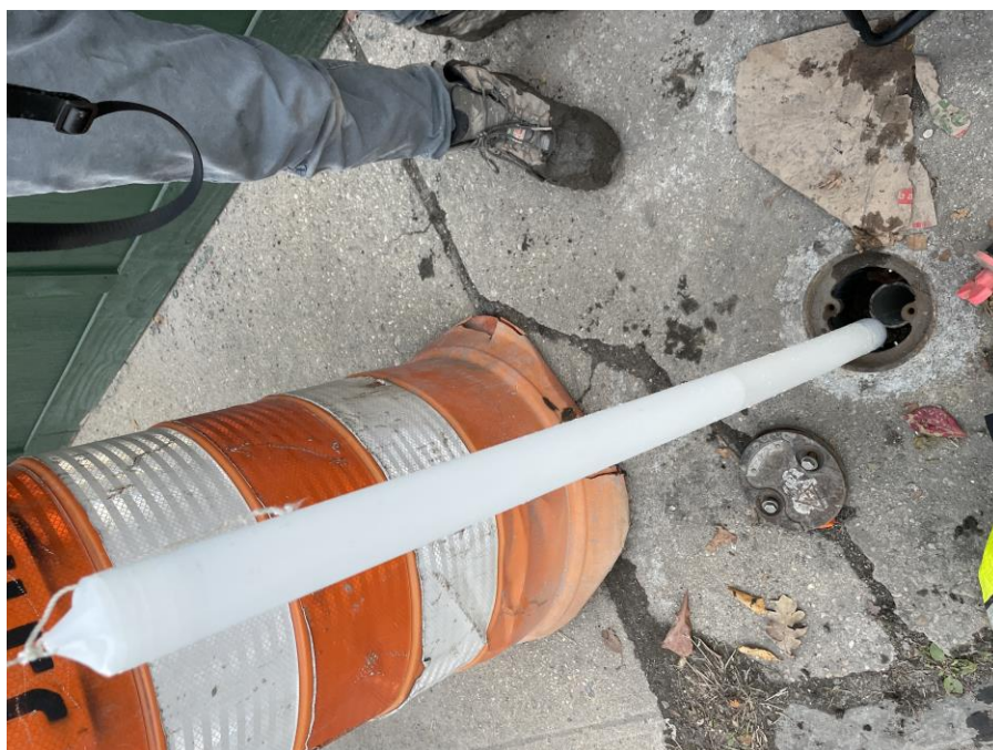
Photo 4: Langan inspecting groundwater conditions at off-site monitoring well MW27
