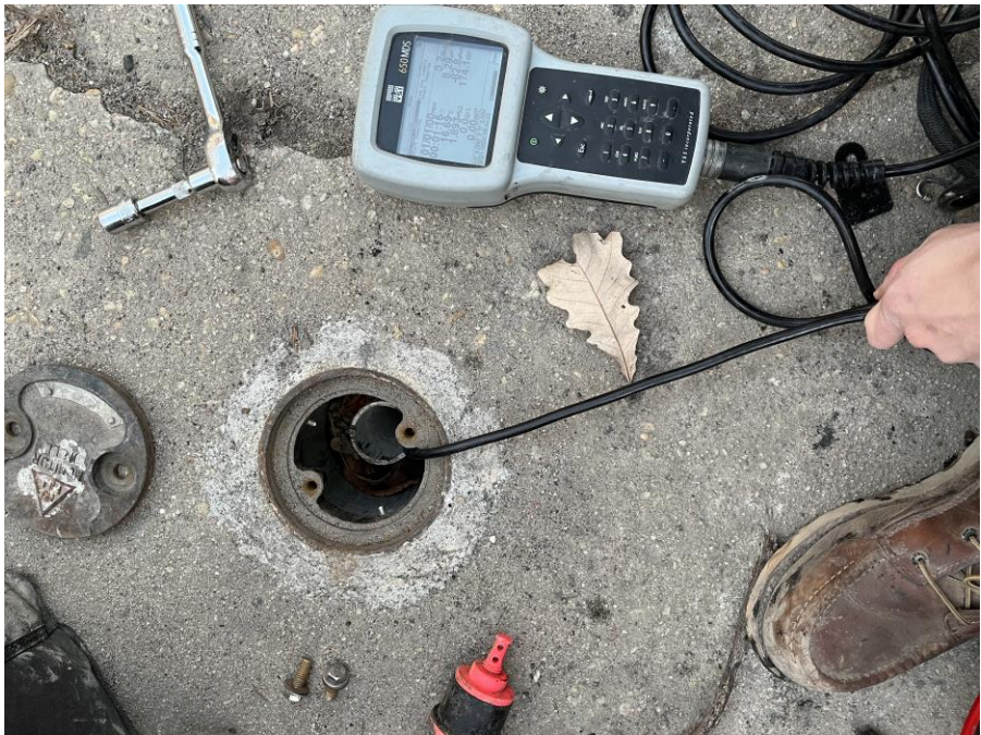
Photo 4: Langan collecting groundwater parameters from off-site monitoring well MW27
