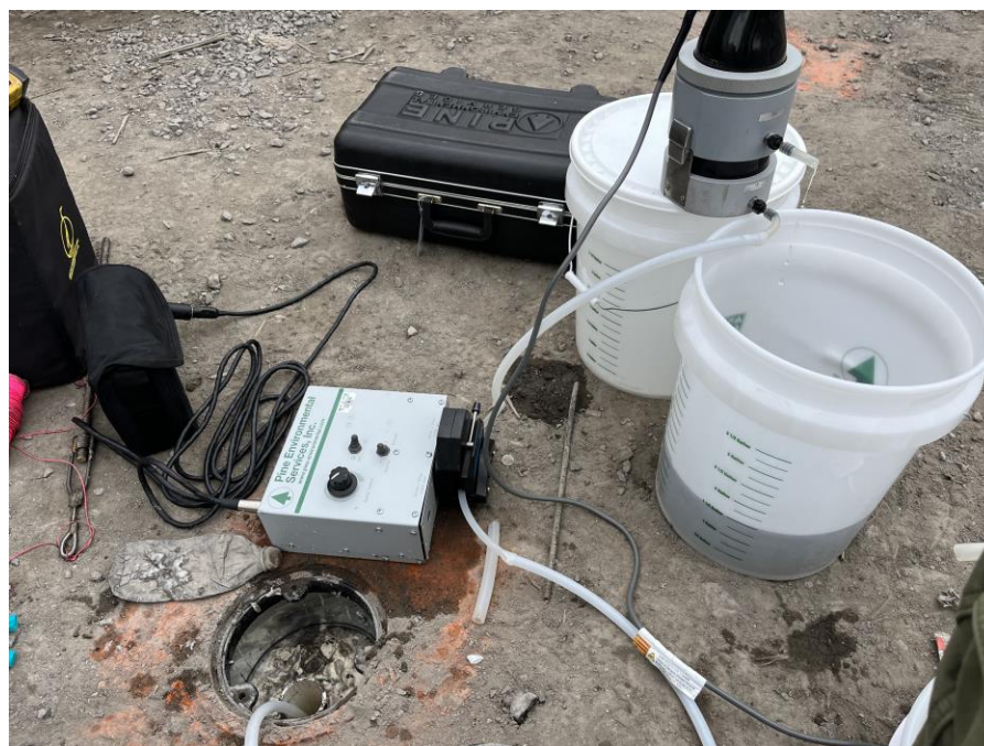
Photo 3: Langan collecting groundwater parameters from monitoring well MW41-N in southeastern part of Sackett Place (facing south)
