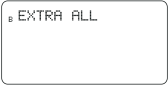
Figure 18: Display showing manual watering, for stations assigned to program B, selected
