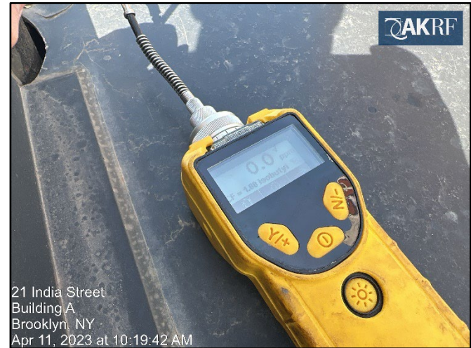
Photograph 8: Exhaust stack sample port PID measurement.
