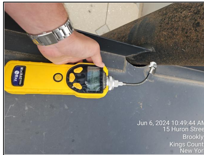
Photograph 6: Exhaust stack sample port PID measurement.
