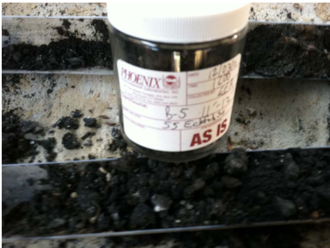
Fig 3. View of soil sample collected from soil boring B-5.
