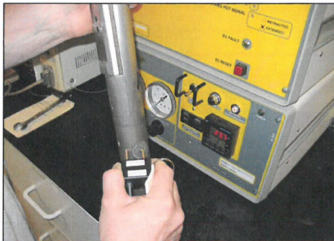
Figure 5.4 Operation of the EC Dipole Test Jig.
