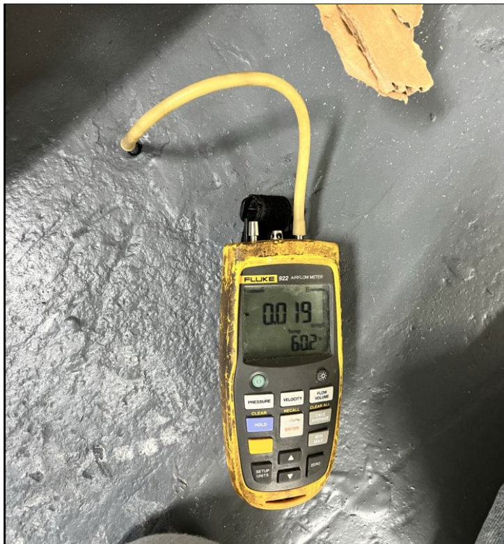
Photograph 5. Fluke 922 Air Flow Meter used for vacuum reading, recording -0.019 iwc at vapor monitoring point PV-3. December 8, 2022.
