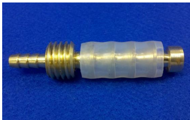
Figure 1. Assembled VAPOR PIN® sampling device
