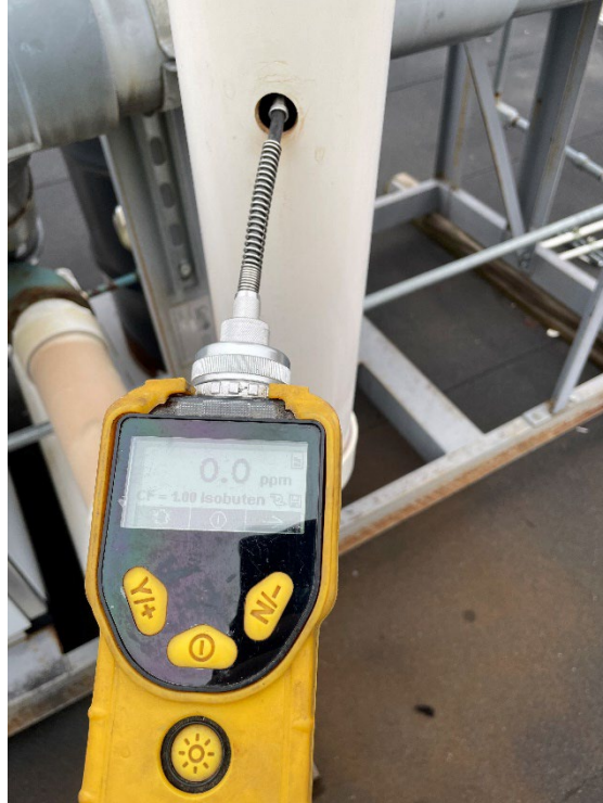
Photo 5: View of PID reading of the effluent air at Blower B discharge stack.
