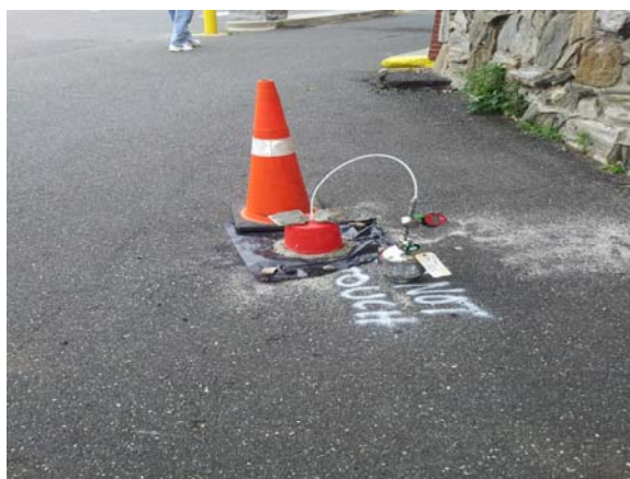
Photo 6: Soil vapor sample point assembly.
