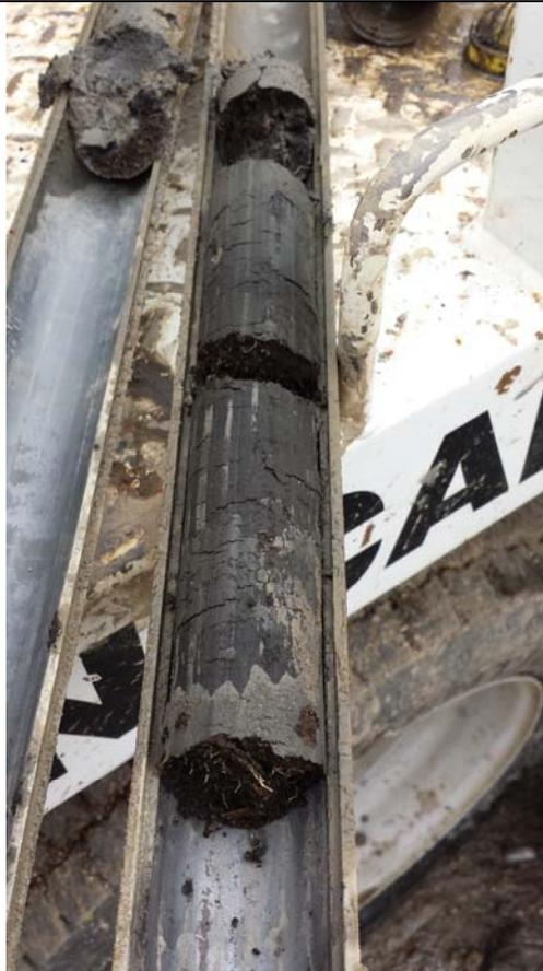
Photo 9 – View of gray fines (fine sand and silt) recovered in all borings from depths ranging from 11 to 30 feet below grade. This material was typically clean (i.e., without visual, olfactory or PID evidence of petroleum impacts).
