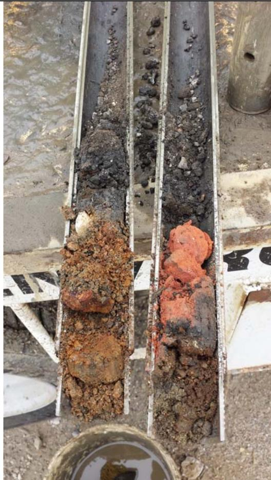
**Photo 7 – View of black-stained soil exhibiting strong odors and PID response collected in a two-foot split-spoon sampler. Petroleum impacted soil was typical in most borings from the surface to four to twenty five feet below grade.**
