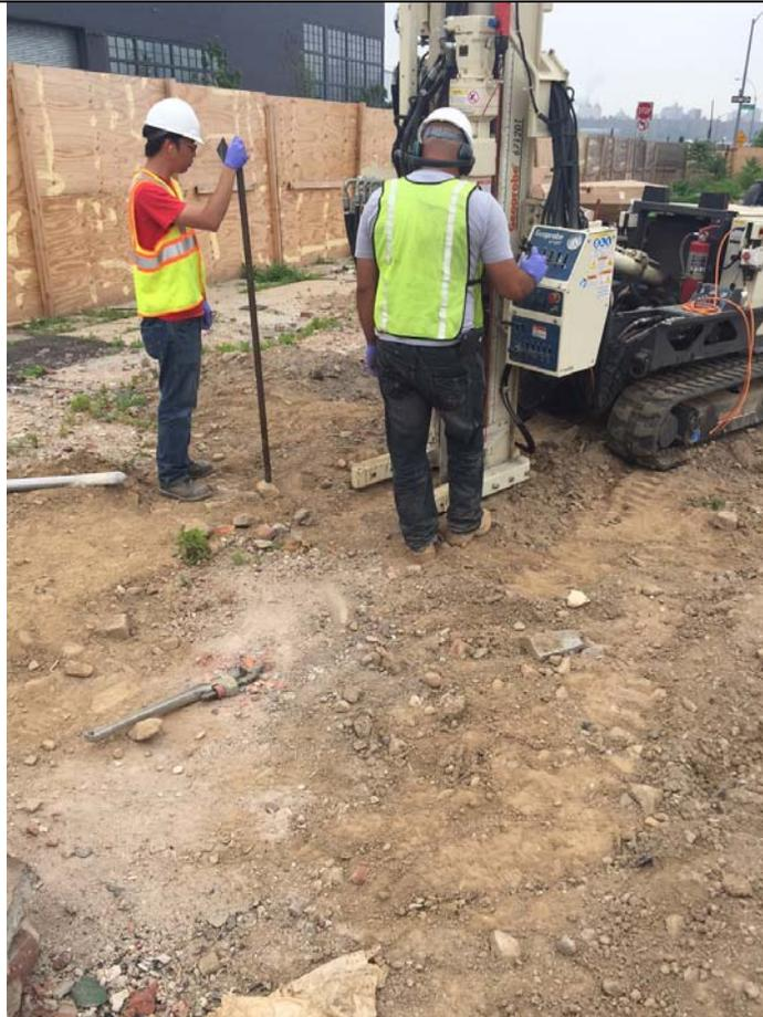
**Photo 5 – Depth to groundwater measurements taken upon completion of borings through the hollow-stem auger sections.**
