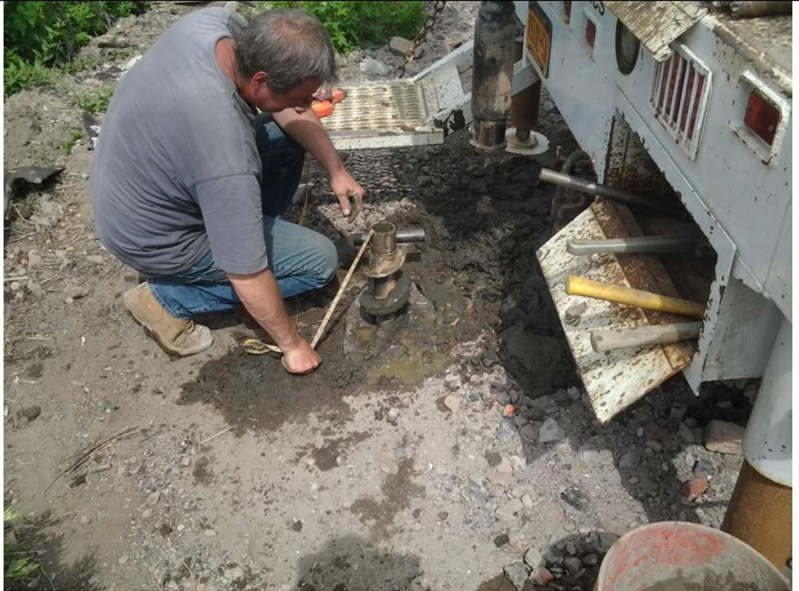
**Photo 6 – View of historic fill material collected in a two-foot split-spoon sampler. Fill material was typical in all borings from the surface to three to ten feet below grade.**
