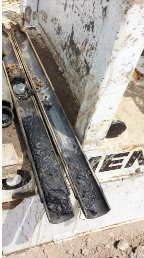
**Photo 8 – View of dark brown peat/compacted organics, recovered at depths ranging from 17-24 feet below grade. Peat was encountered in most borings installed. Specifically, those on the western side of the Site.**
