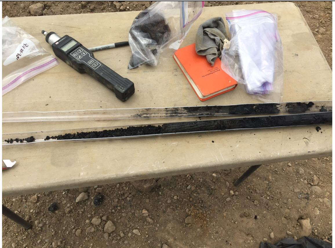
**Photo 11 – View of all soil boring intervals collected in five foot long sleeves using Geoprobe. Soil recovered was inspected for visual, olfactory and PID evidence of petroleum impacts.**
