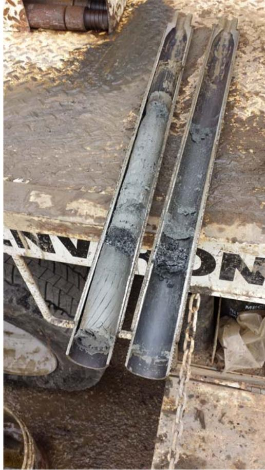
Photo 10 – View of black-stained soil exhibiting strong odors and PID response collected in a five foot sleeve using Geoprobe. Soil recovered was inspected for visual, olfactory and PID evidence of petroleum impacts.
