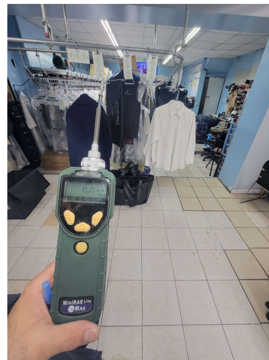
Organic vapor survey on 1 st floor
